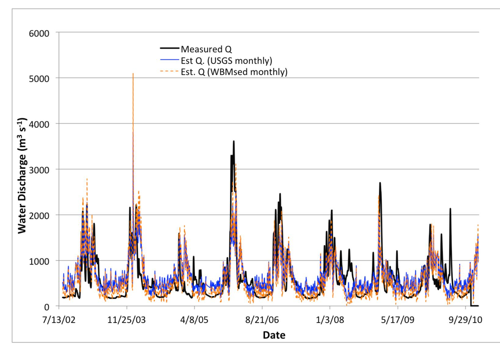
Satellite discharge measurements for a site on the Willamette River in north-west USA using modelpredicted (orange) and gauged (blue) discharge as calibration. Gauged discharge from a colocated USGS station is the black line.
