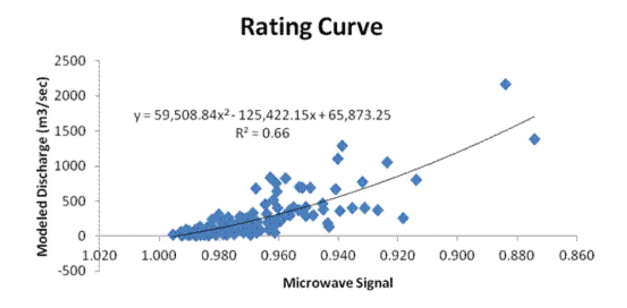
Plot of microwave discharge estimator signal for a site on the White River USA (site number 516) versus WBMpredicted monthly daily mean, max and min discharge. Without groundbased information, we calibrate the remote sensing signal to discharge.
