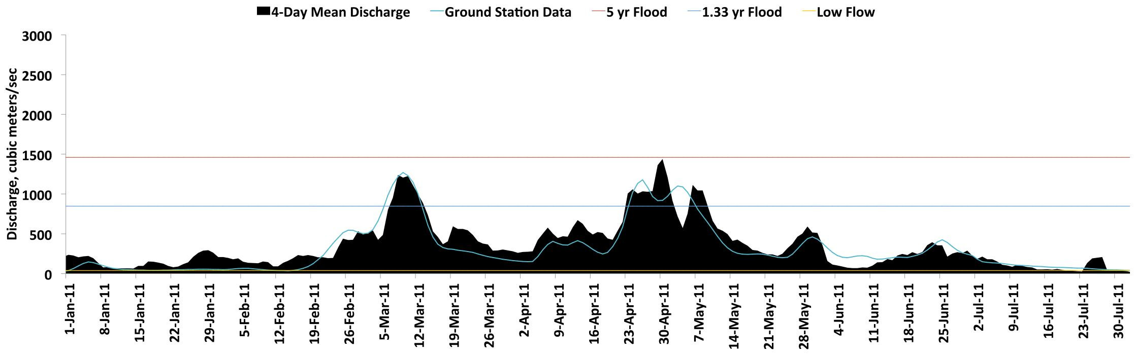
River discharge measurements (black) for a site on the White River, southern Indiana, USA using model-predicted discharge as the rating curve calibration (no ground-based information was used). The blue line is gauged discharge from a co-located gauging station (USGS 03360500 White River at Newberry, IN).
