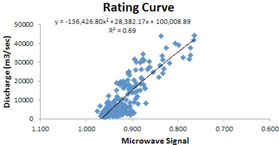
**Figure 4.** Sample calibration/rating curve (site #1936, Brahmaputra River) comparing the TRMM 37 GHz discharge estimator to WBM hydrology model-estimated discharges. The model was run in one day increments for 2001-2005; the plot compares monthly mean, maximum and minimum values for those years for both signal and modeled discharge. The same technique provided the rating curves for the plots shown in Figure 2.
