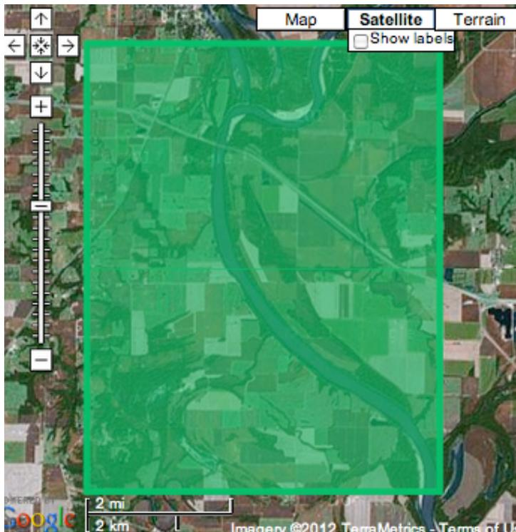
**Figure 3.** View of the measurement site for the Figure 2 plots (satellite gauging site #91). Microwave emission from this pixel is ratioed to brightness values obtained within a 7 x 7 pixel array centered on this pixel<sup>7,8</sup>, thereby removing most daily and seasonal variations due to non-hydrological factors.
